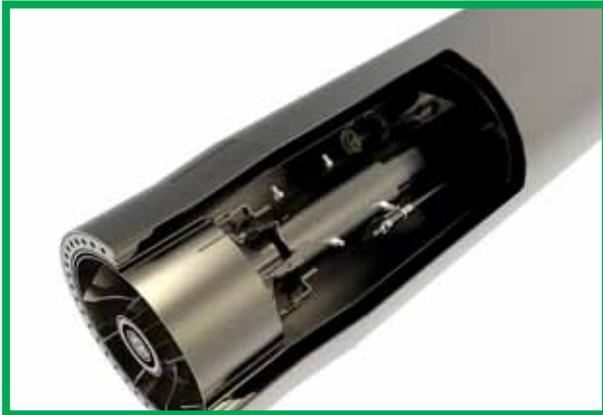
Multi-fuel burner tip: Equipped with lances for liquid and slurry fuels in the center. Surrounding the center there are channels for gas, solid fuels, and air. It also houses the swirl turbulator.
